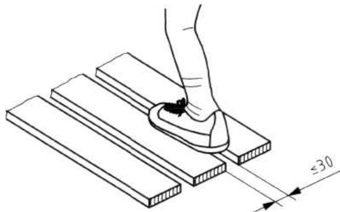
**7.17 Crushing or smashing points.** Crushing or smashing points occur in a situation where movable elements are assembled too close to each other, or too close to permanent elements in such a way that they create changeable cracks which can be reduced to zero under load. Presence of such points is usually signalled by characteristic wearing through of materials. Presence of smashing point can cause such accidents as cutting of fingers or serious fractures in case of the crushing point.
