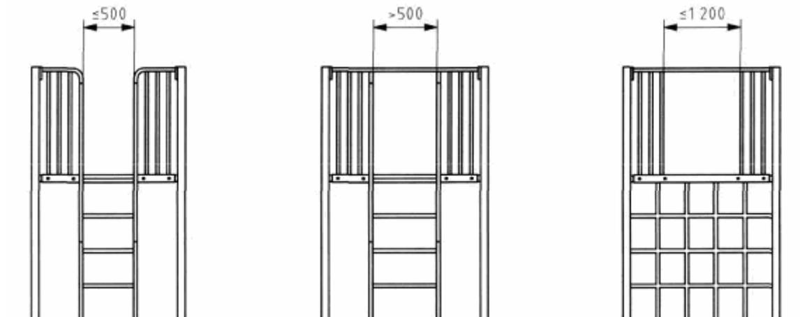
**8.8 Suitable guardrails.** Shields used as an exclusive way of protection against fall should be used only in devices which are hard to approach with the free fall height between 1 and 2 meters. Shields do not protect the user passing under. The shields should be assembled on the height of 600 – 850 mm from the platform.
